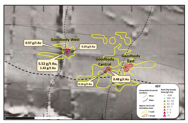
**Figure 1.** Location of recent rock chip samples (triangles) within the Goodbody gold prospect area. The Goodbody West to Goodbody Central mineralized quartz vein zones are hosted within a 1.5 km stretch within the broader 3km long Goodbody Au soil anomaly. Overlaid on greyscale Total Magnetic Intensity (TMI)1VD basemap and satellite imagery.
