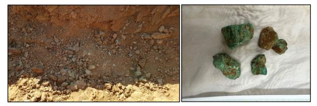
Photo 1: Copper-oxide (malachite) mineralisation in surface excavation and malachite rich rock chips at Browns prospect
