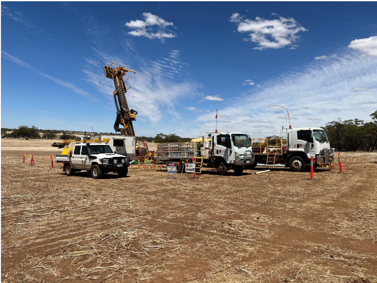
Figure 6: Diamond drill rig at Manning prospect
