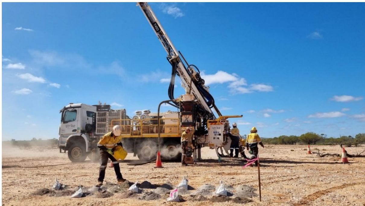
Figure 4: AC drill rig at Browns prospect
